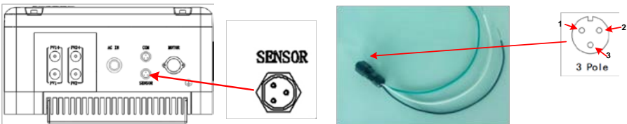
Figure6-5 Water level sensor interface define
